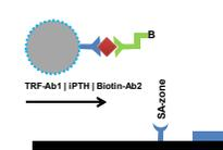
Figure 8: TRF Lateral Flow assay format. TRF-Ab1 and Ab2-bt form a sandwich with iPTH which is then captured by the streptavidin line.
