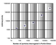
Figure 3A: TRF particles interrogated in a Perkin Elmer AlphaScreen. Data plotted is the result from three runs.
