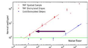
Figure 5: Comparison of TRF label to a 40nm gold Colloid label. TRF label read with CC low cost reader, gold colloid read using Hamamatsu ICA1000 reader. Substrate used lateral flow membrane
