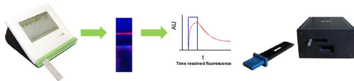
Figure 1: Second (left) and third (right) generation integrated low cost readers with rich UI and wireless connectivity. At the core of which is a high sensitivity label and detection technology that can measure both fluorescence and phosphorescence. The unique way in which the measurement is made enables significant sensitivity enhancements over both traditional labels and amplification techniques
